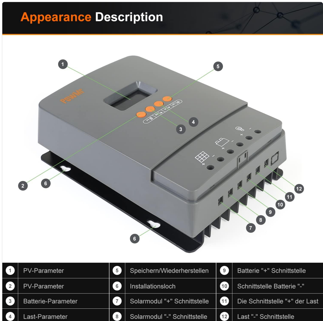
Figure 3.2.1: Controller Components
