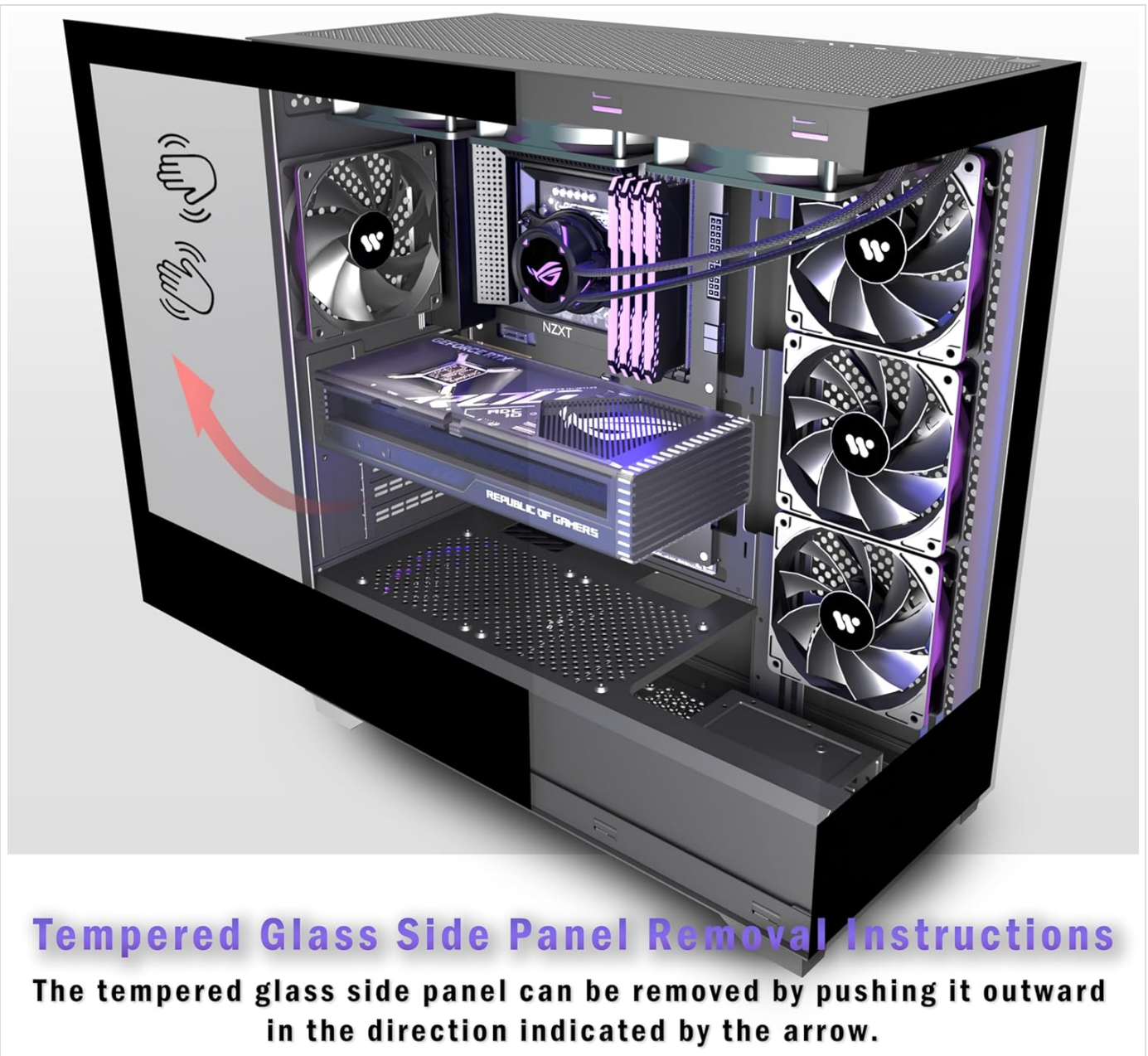
Figure 3.1.1: Tempered Glass Side Panel Removal. This image illustrates the method for removing the tempered glass side panel by pushing it outwards, revealing the interior of the PC case.
