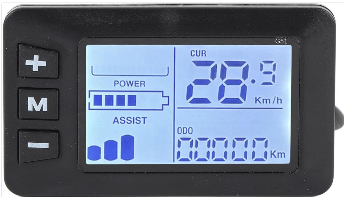
Figure 4.1: Close-up view of the G51 LCD Display screen. The screen clearly shows "CUR" (current speed) at 28.9 Km/h, "ODO" (odometer) at 00000 Km, a battery "POWER" indicator, and an "ASSIST" level bar graph. The "G51" model designation is visible in the top right corner.
