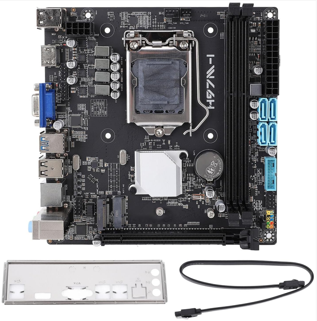
Figure 3: Yoidesu LGA1150 ITX Motherboard with included accessories. The motherboard is displayed alongside its included accessories: an I/O shield and a SATA data cable.
