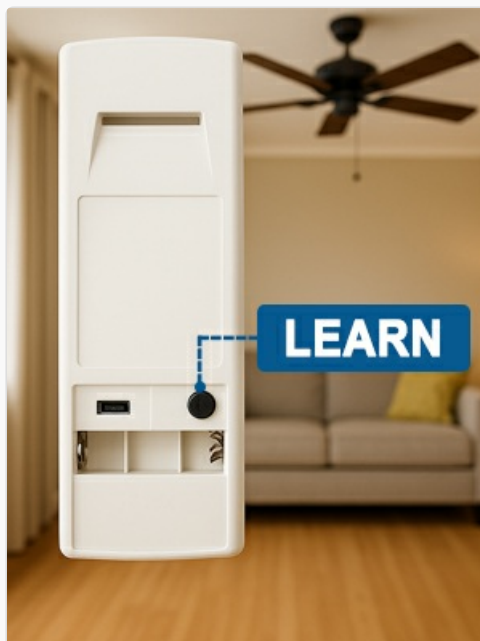
Figure 6: Location of the 'LEARN' button on the back of the remote for pairing.
