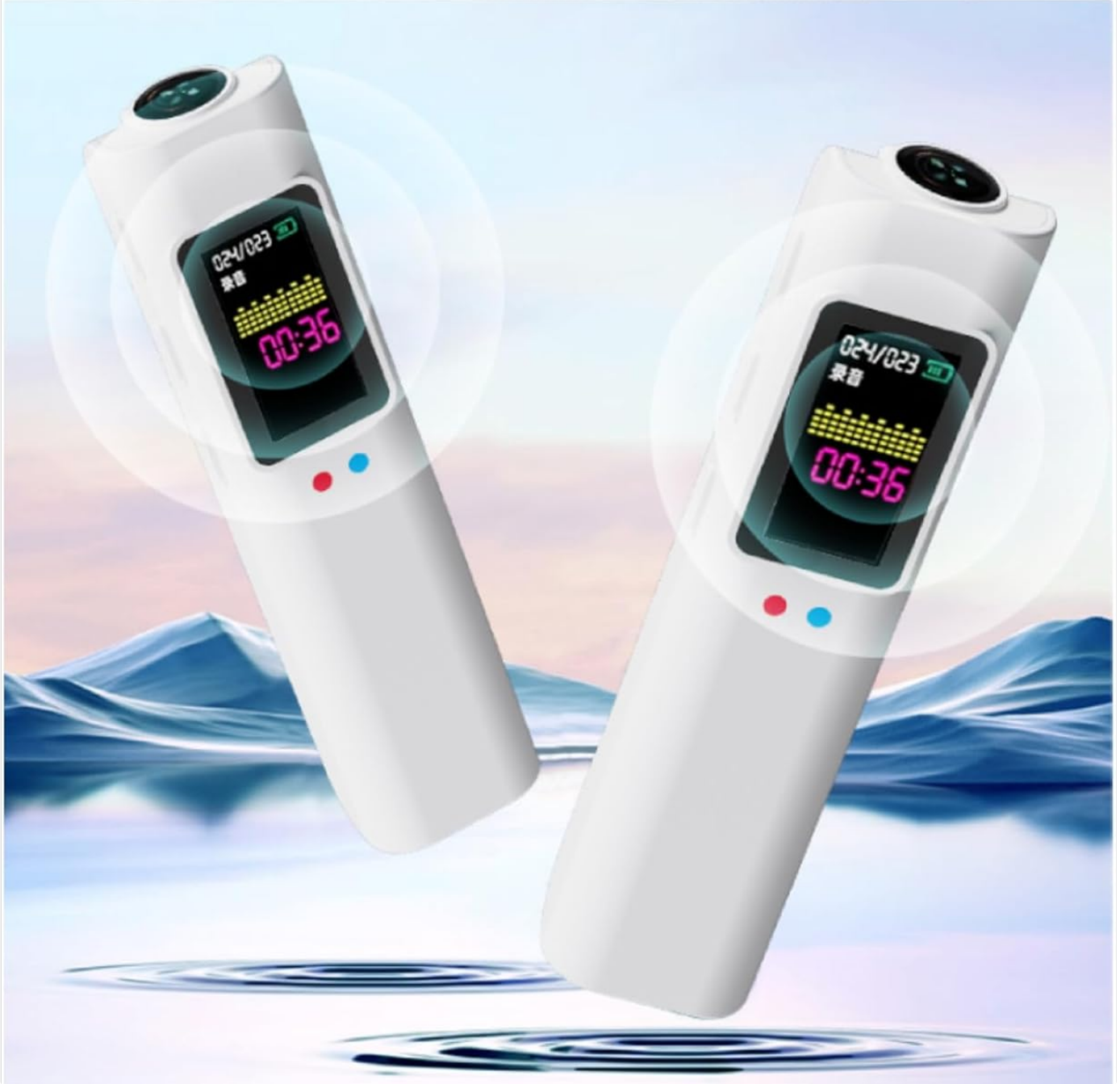
Figure 4.4: The 0.96-inch IPS color screen displaying a live view, with side physical buttons for operation.
