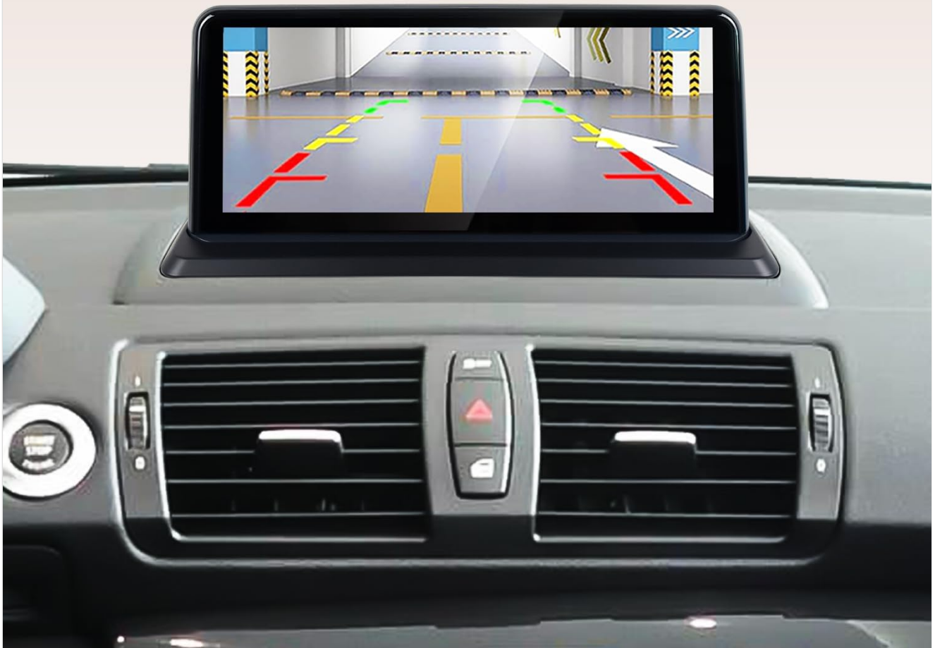
Figure 6: Reverse camera view displayed on the screen with parking guidelines.
