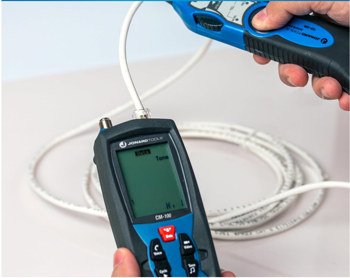
Image: The CM-100 Cable Mapper Pro connected to a network cable, with an RJ45 identifier visible, illustrating the compatibility and function of the system.
