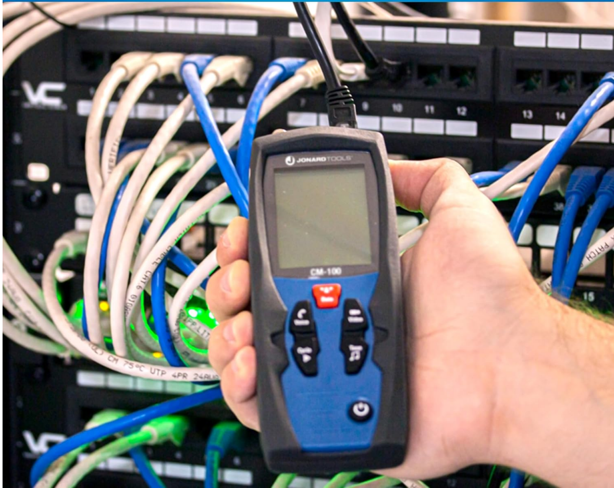
Image: A technician using the CM-100 Cable Mapper Pro to test a network cable connected within a server rack, demonstrating cable mapping in a live environment.
