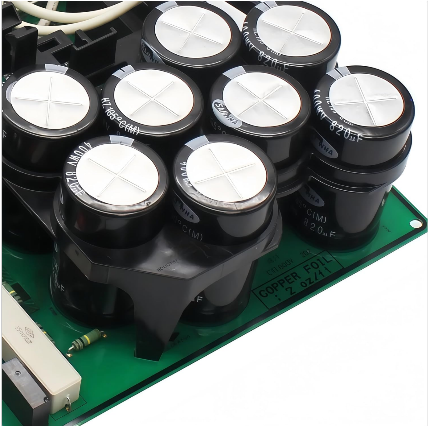
Figure 6.1: Close-up view of the power capacitors on the PCB, critical for stable power delivery.
