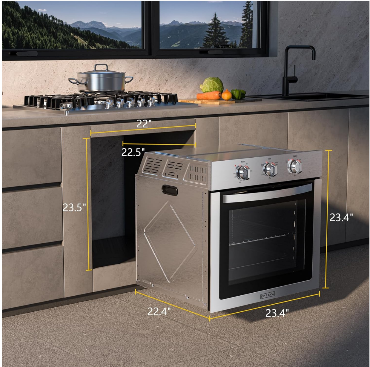
Image: Diagram showing the external dimensions and required cutout dimensions for the Empava 24-inch Electric Single Wall Oven.
