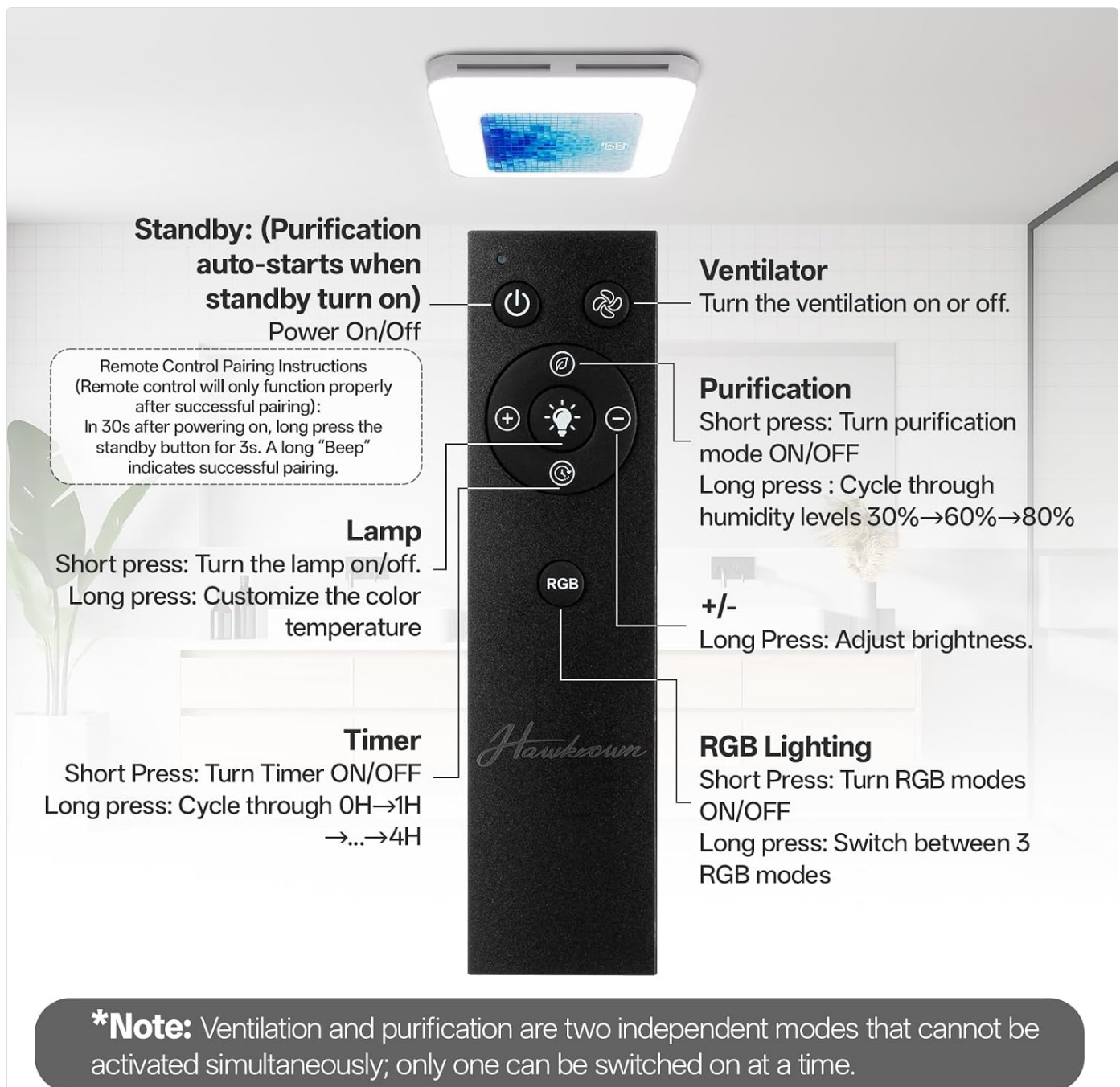
Figure 6.1: Remote control functions overview.
