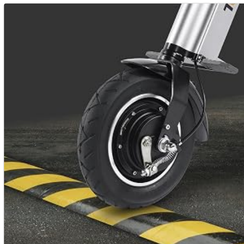
Figure 8: Detail of the durable, explosion-proof pneumatic tires.
