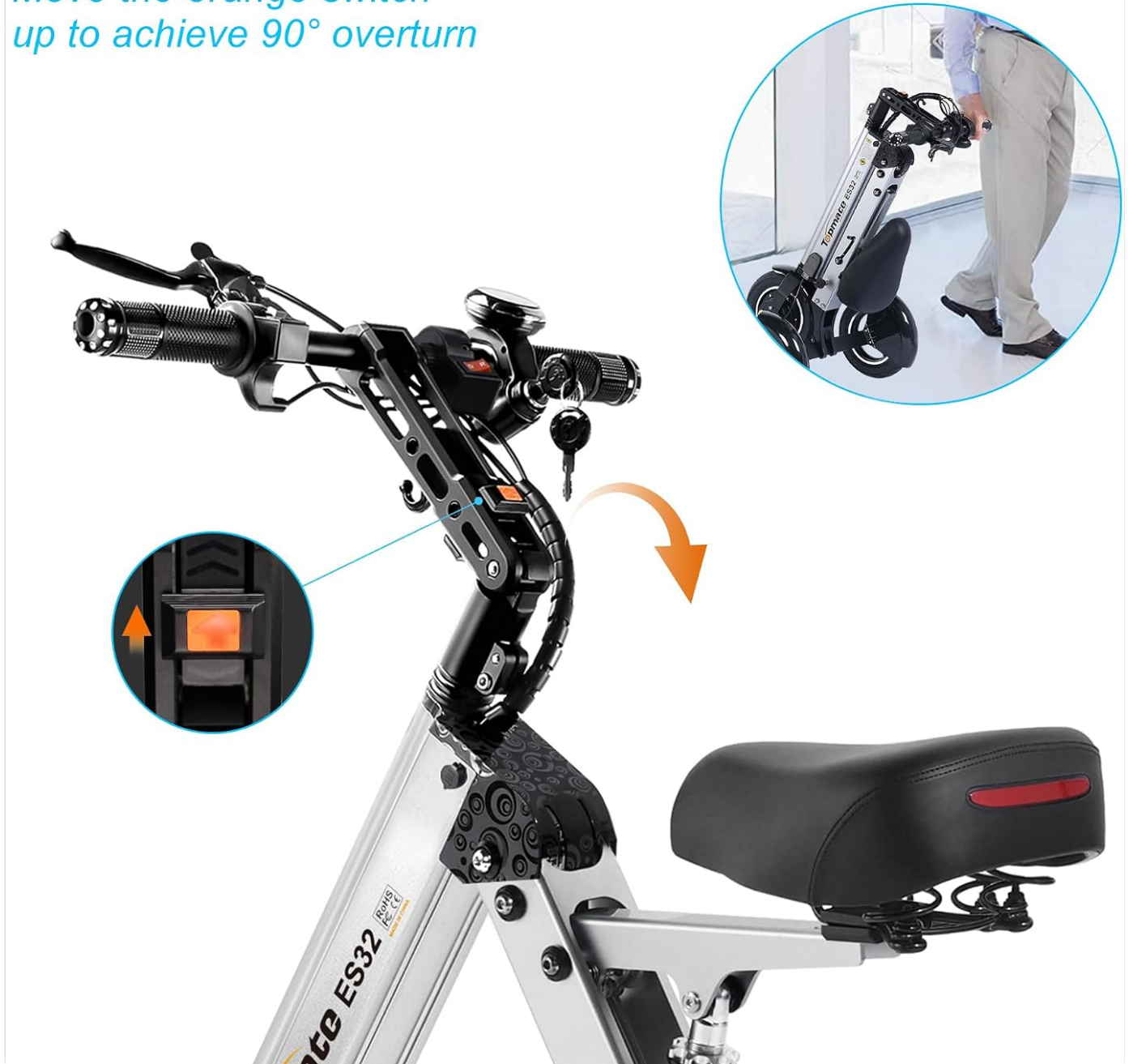
Figure 2: Detail of the orange switch for unfolding the scooter.
