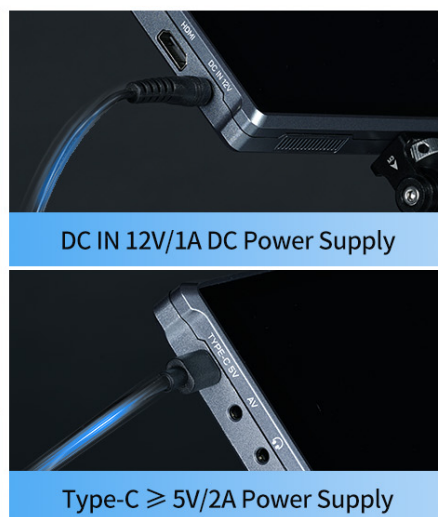
Image: Versatile power options for the monitor, including NP-F series battery, DC 12V input, and Type-C 5V input.
