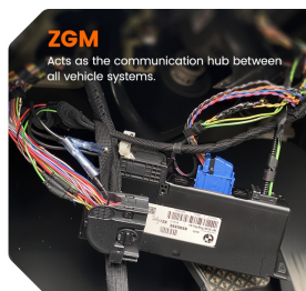
Image: Details on CAS (Car Access System) and ZGM (Central Gateway Module) functions.
