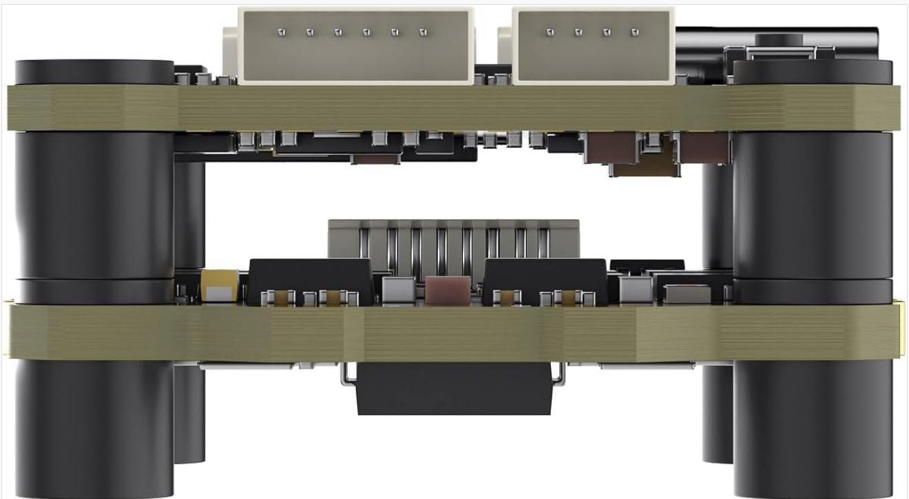
Figure 3.3: Side view of the stack, showing the separation between the flight controller and ESC boards.
