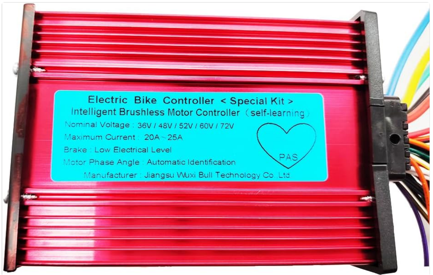
Image: Close-up view of the controller unit's label, detailing specifications such as nominal voltage (36V/48V/52V/60V/72V), maximum current (20A-25A), brake type (High/Low Electrical Level), and motor phase angle (Automatic Identification).
