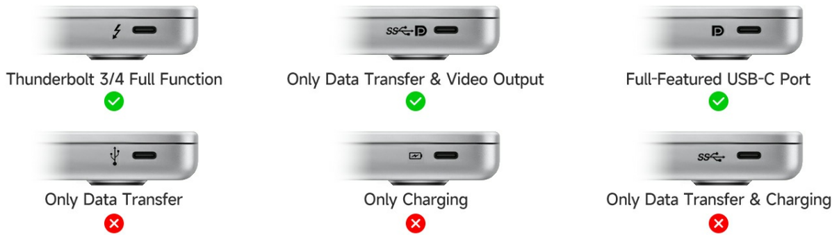
Image: Guide to compatible USB-C port types for video and data.
