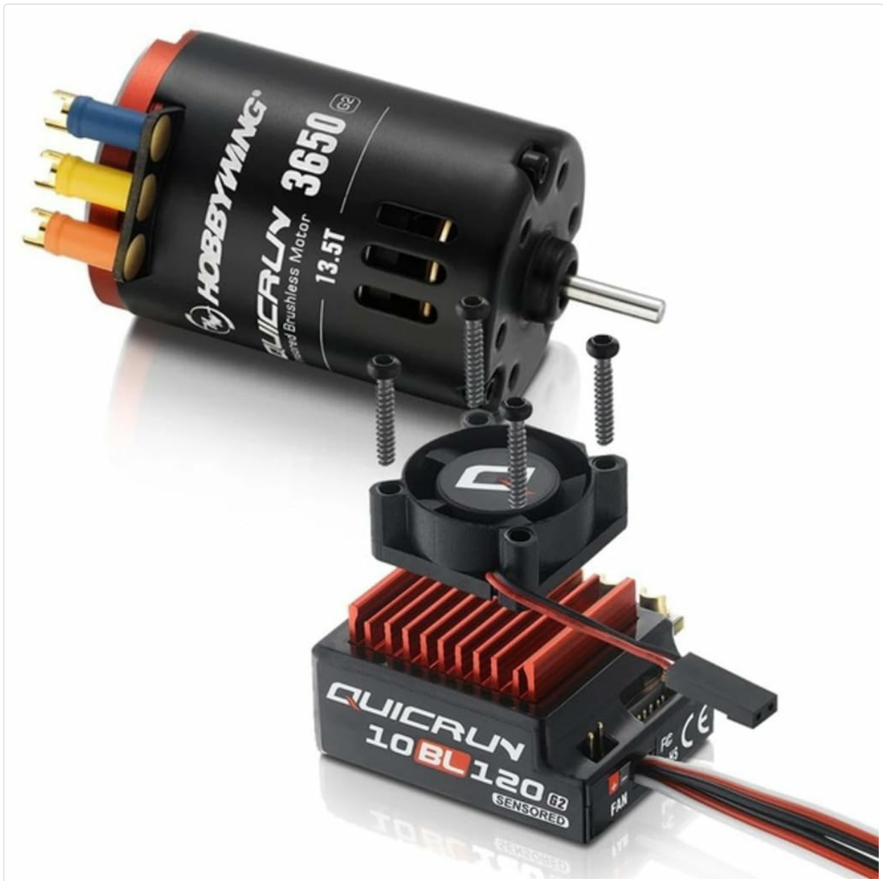
Image: The Hobbywing QUICRUN WP 10BL120 SD G2 ESC and 3650 SD G2 Motor Combo, showcasing the electronic speed controller and brushless motor components.
