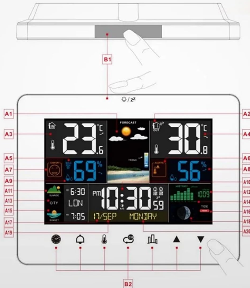
Figure 4.1: Diagram illustrating the touch-sensitive areas (A1-A20, B1-B2) and display segments of the weather station for interaction.
