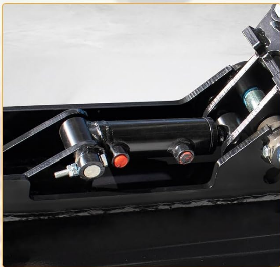
Figure 1: Detailed view of the hydraulic cylinder and pin connections for the tilting bucket. This image highlights the robust construction and the points where the attachment connects to the excavator arm and hydraulic system.
