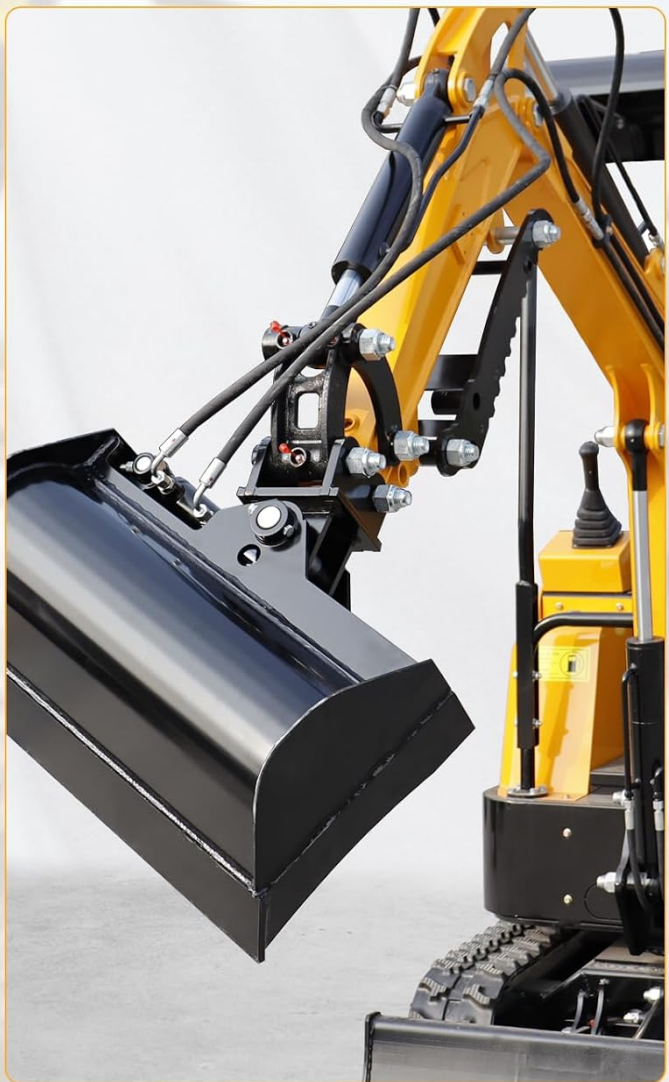
Figure 1: Detailed view of the hydraulic cylinder and pin connections for the tilting bucket. This image highlights the robust construction and the points where the attachment connects to the excavator arm and hydraulic system.
