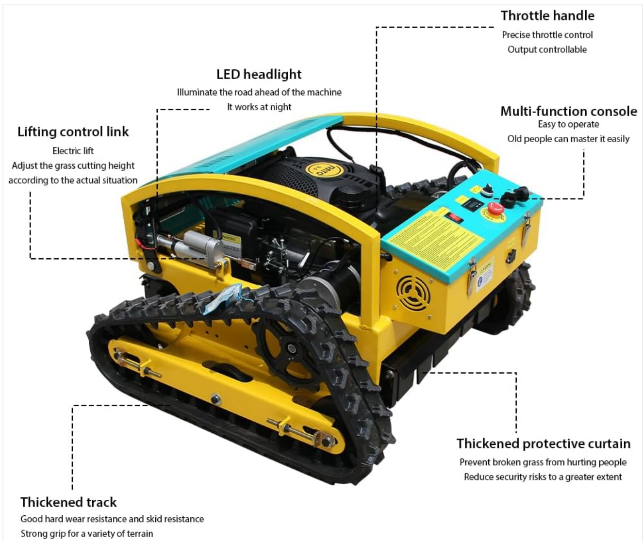
Figure 6: Key components requiring regular inspection and maintenance.
