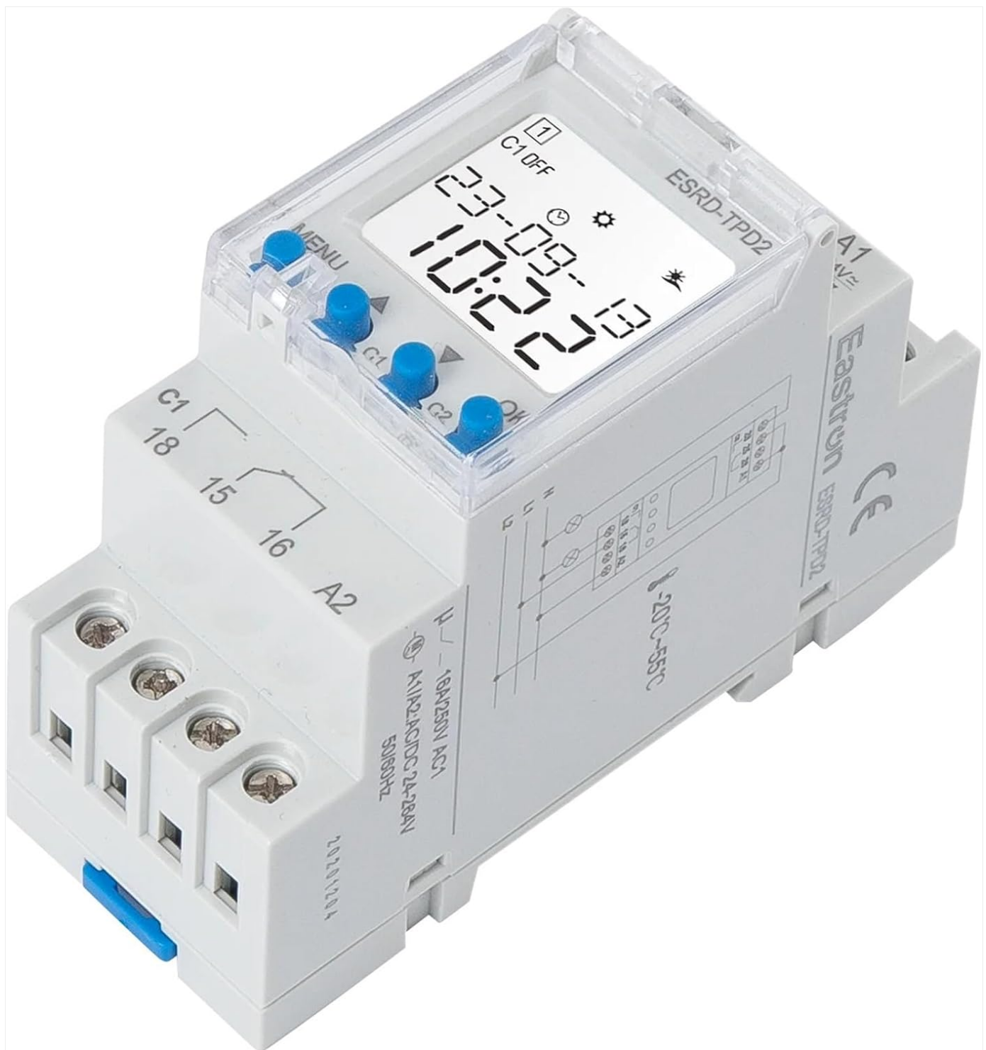
Figure 2: Angled View of ESRD-TPD2. This image provides an angled perspective of the time switch, revealing its compact DIN rail mountable form factor. The side of the device shows additional technical specifications and certifications. The screw terminals for power input (A1, A2) and the two independent output channels (C1 and C2) are clearly visible, along with their respective common, normally open, and normally closed contacts.
