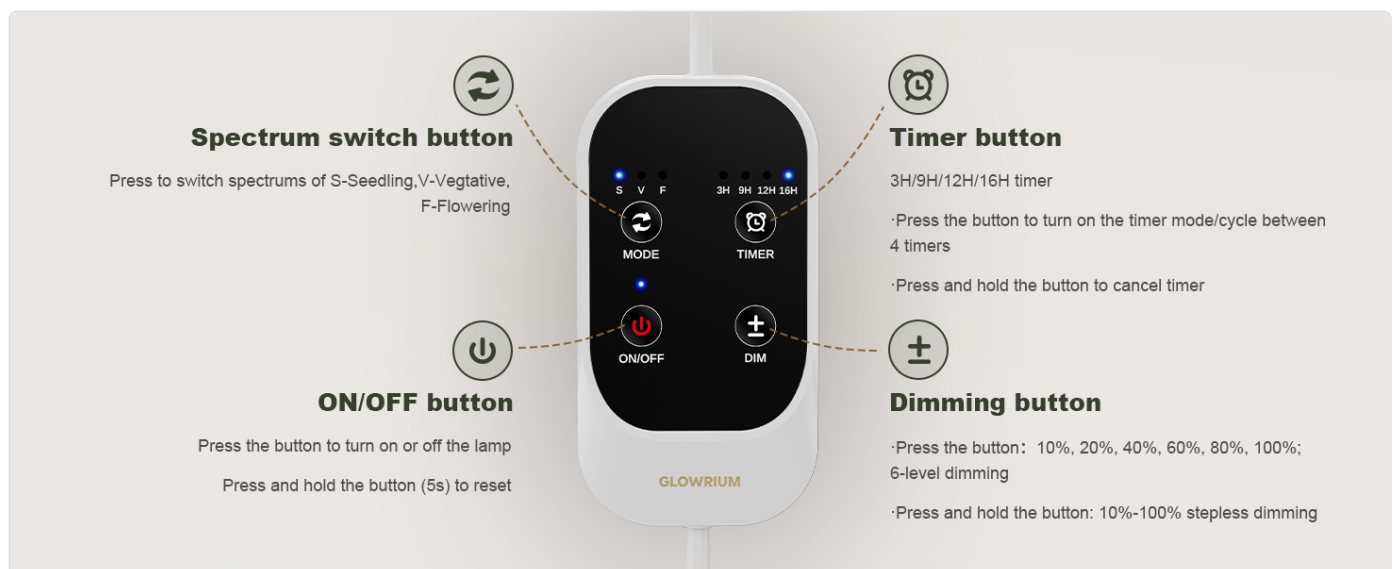
Figure 5.1: Inline Controller Functions
