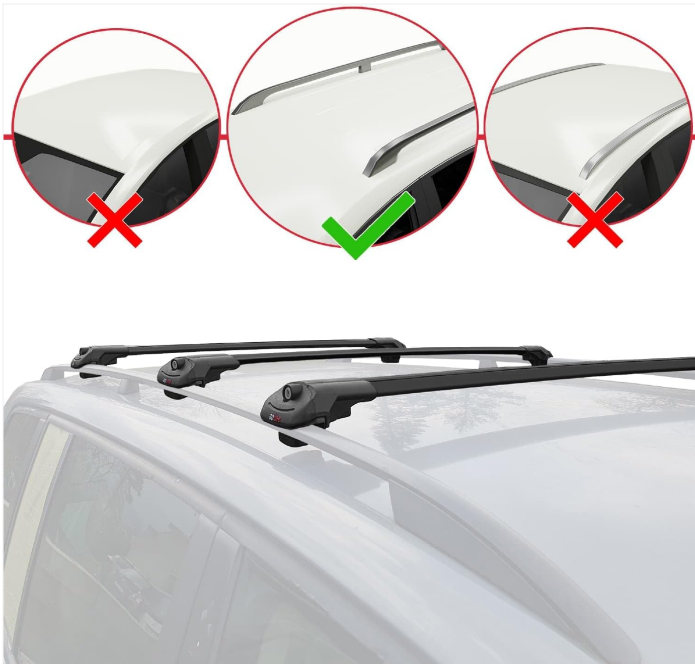
Image 3.1: Visual guide for roof rail compatibility. The ACE-1 system is compatible only with vehicles featuring raised roof rails, as indicated by the green checkmark.
