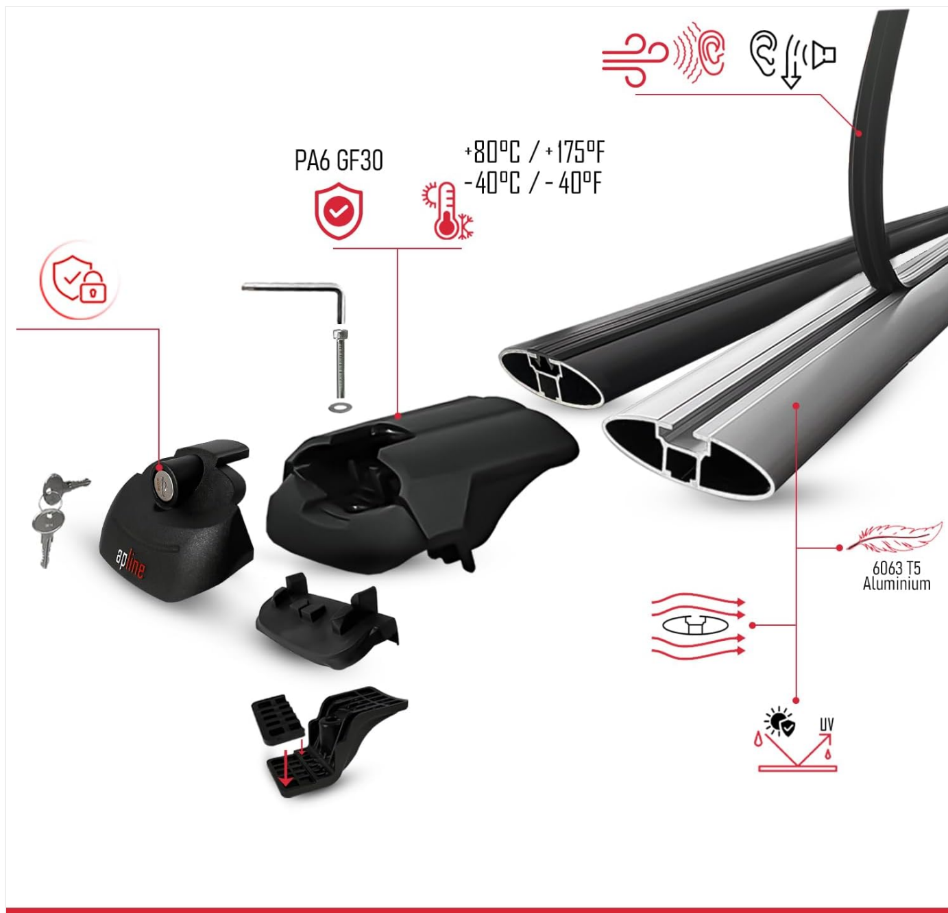
Image 3.2: Detailed view of the ACE-1 components, highlighting the 6063 T5 Aluminum bars and PA6 GF30 plastic parts. It also shows the temperature resistance from -40°C to +80°C and aerodynamic design features.
