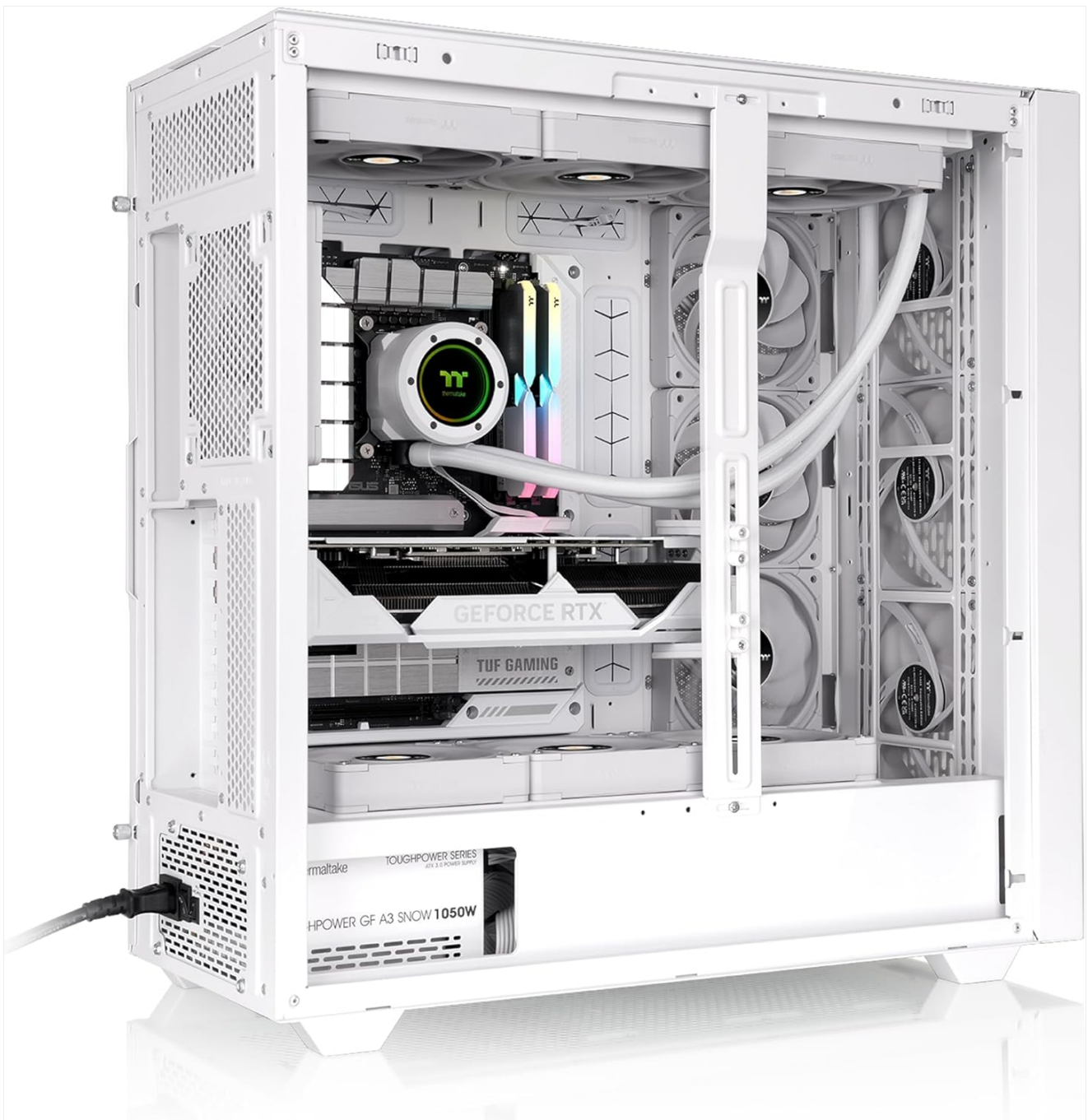
Figure 5.1: An example build showing a graphics card installed and supported by the adjustable GPU brace within the chassis.
