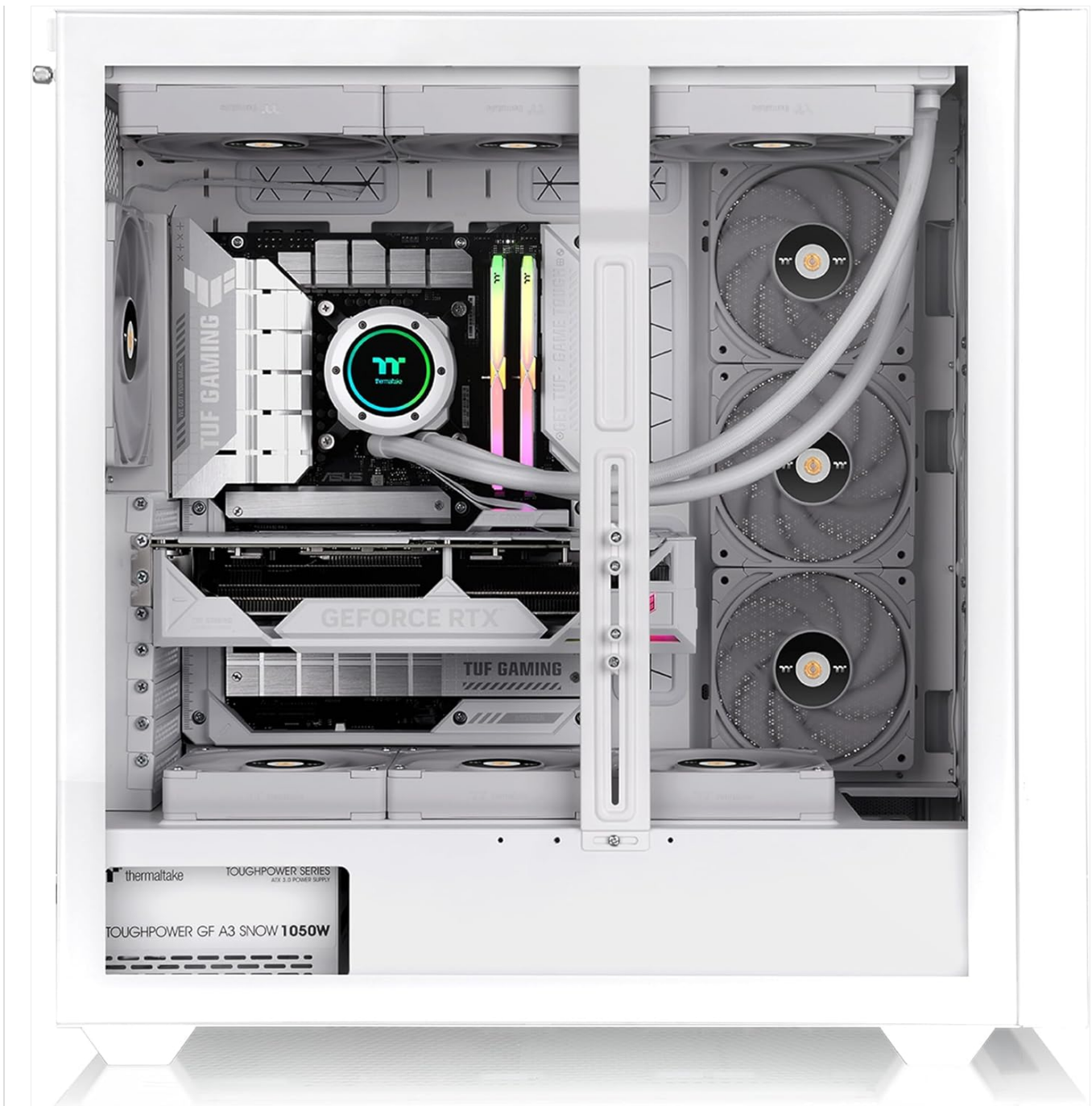
Figure 5.2: A top-down interior view of the chassis with cooling components installed, demonstrating potential fan and radiator placements.
