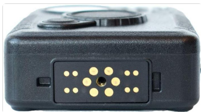
Bottom View: Shows the contacts for connecting to the docking station.
