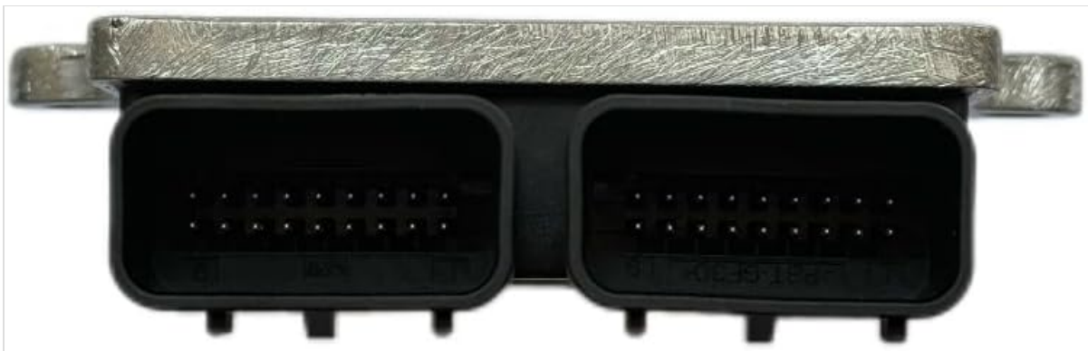
Figure 4.1: View of the dual 36-pin connectors on the WKNYSYK CDI ECU Controller. This image highlights the two electrical connection points for vehicle integration.
