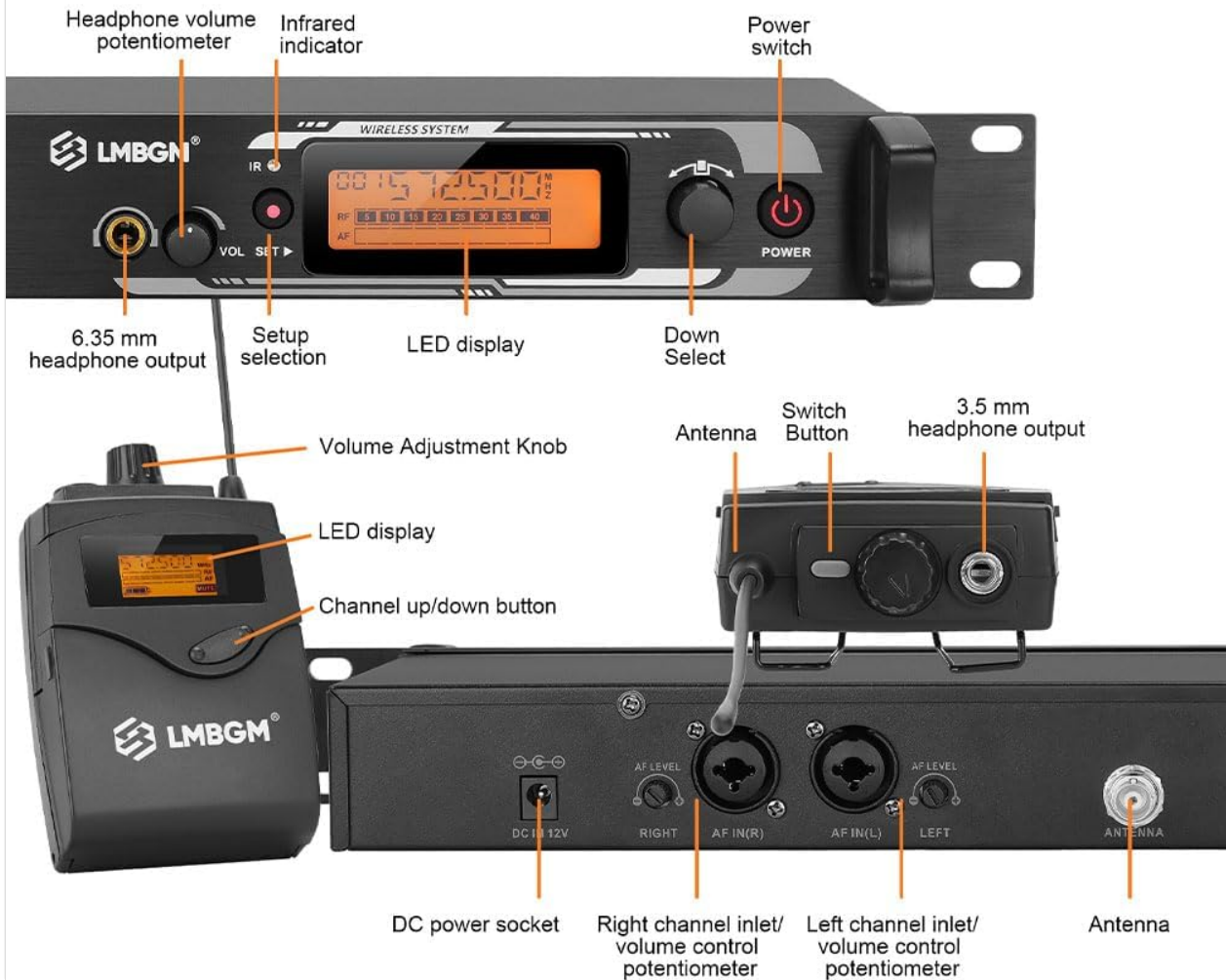
Figure 2.3.1: Detailed view of the front panel controls (headphone output, volume, setup, LED display, power switch) and rear panel connections (DC power, AF input, antenna) of the transmitter, along with the bodypack receiver's volume and channel controls.
