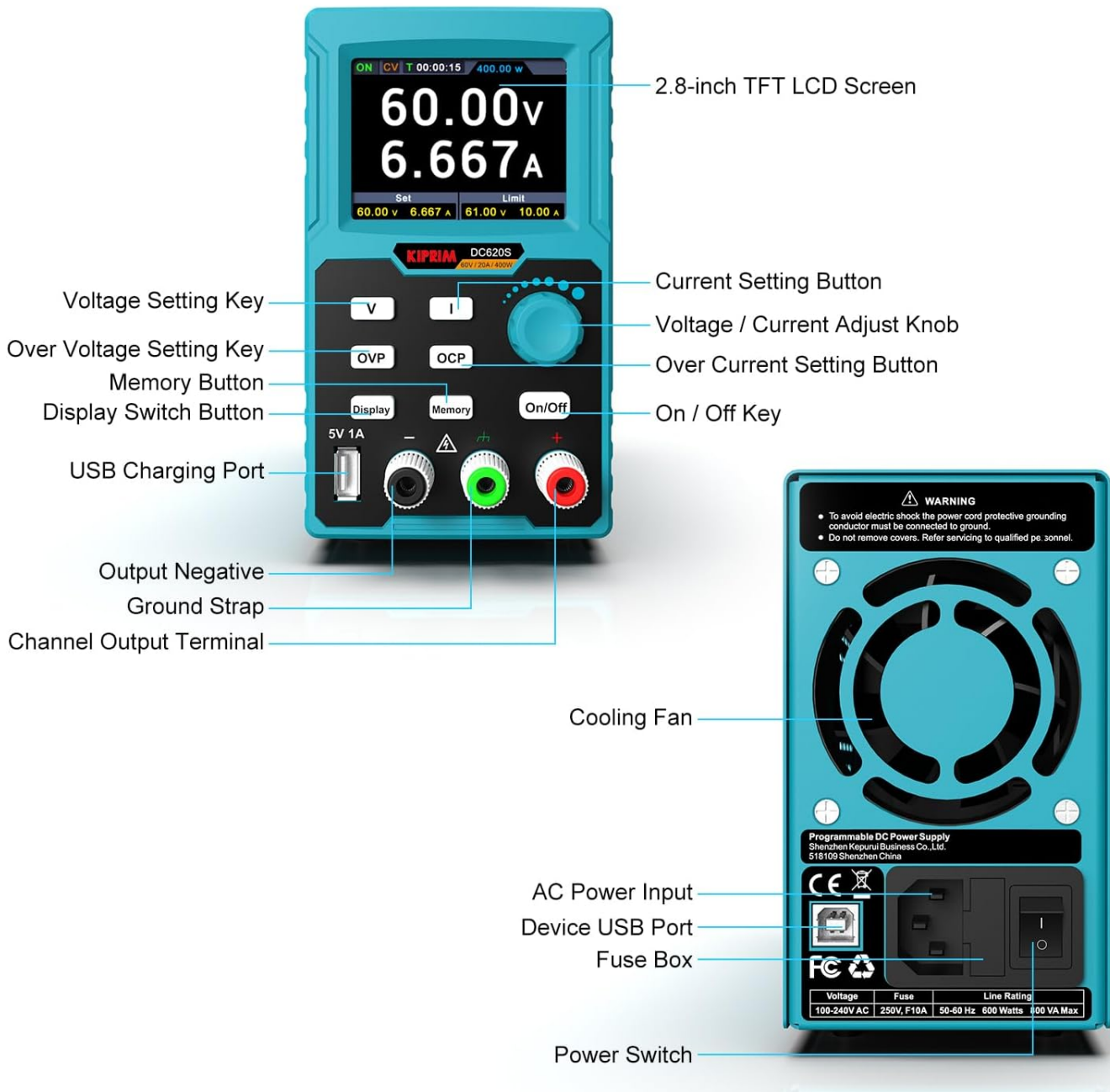
Figure 3: Front and rear panel components and their functions.
