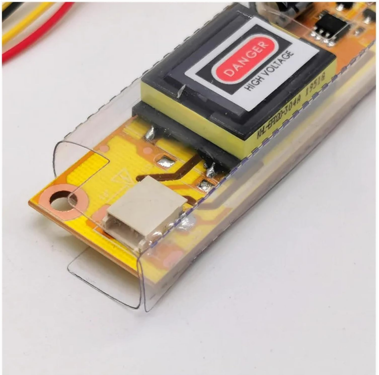
Image: The inverter board, showing a 'DANGER HIGH VOLTAGE' label, which powers the LCD backlight.
