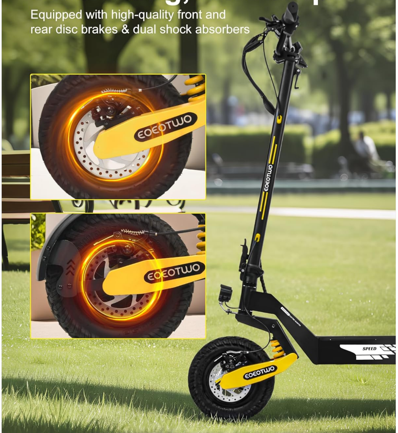
Figure 3.3: The scooter is equipped with high-quality front and rear disc brakes and dual shock absorbers for safe and comfortable riding.
