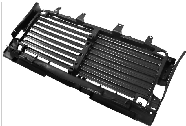
Figure 4: Angled perspective of the active grille shutter with blades closed.
