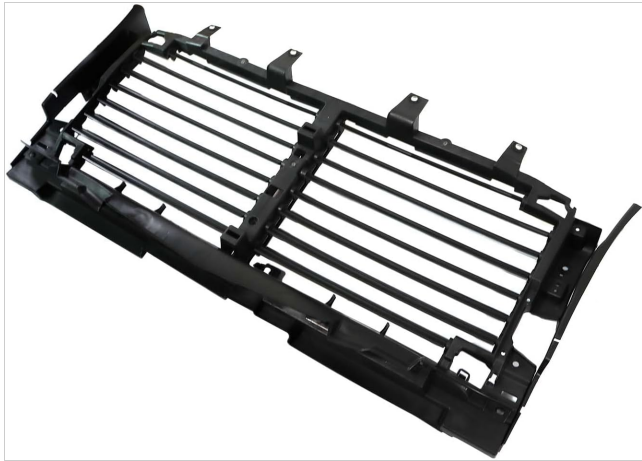
Figure 3: Angled perspective of the active grille shutter with blades open.
