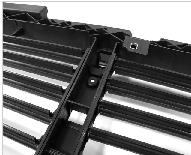
Figure 7: Detailed view of the internal mechanism of the active grille shutter.
