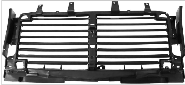
Figure 1: Front view of the active grille shutter, showing the blades in an open configuration.
