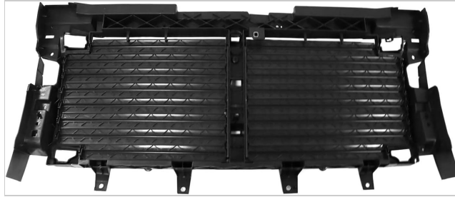
Figure 5: Rear view of the active grille shutter, showing the reverse side of the closed blades.
