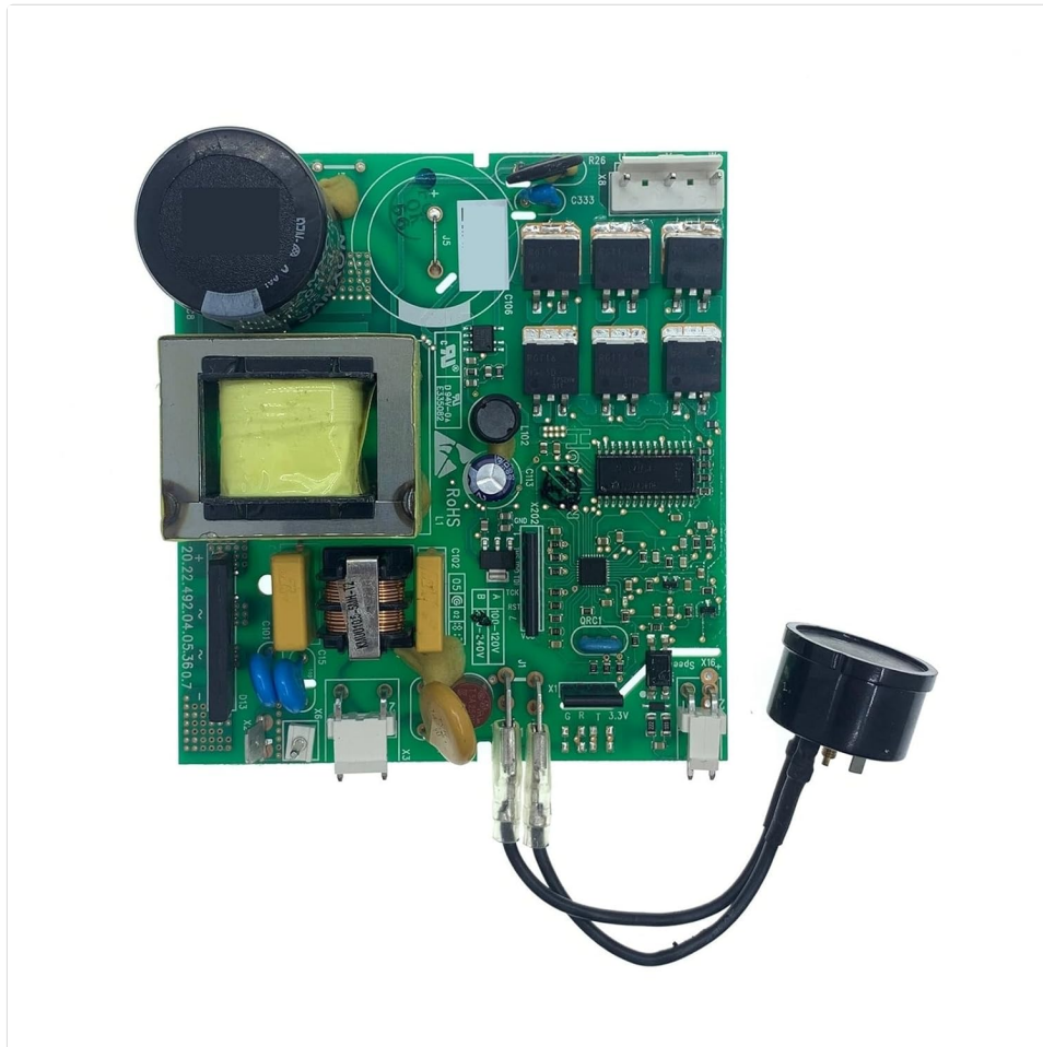
Figure 1: Front view of the DONPER VFL110CY1 Refrigerator Compressor Inverter Drive Control Board. This image displays the front side of the control board, showing the main components including the large capacitor, transformer, and various integrated circuits. The board is green with white markings, and a connected sensor or component with black wires is visible on the right.
