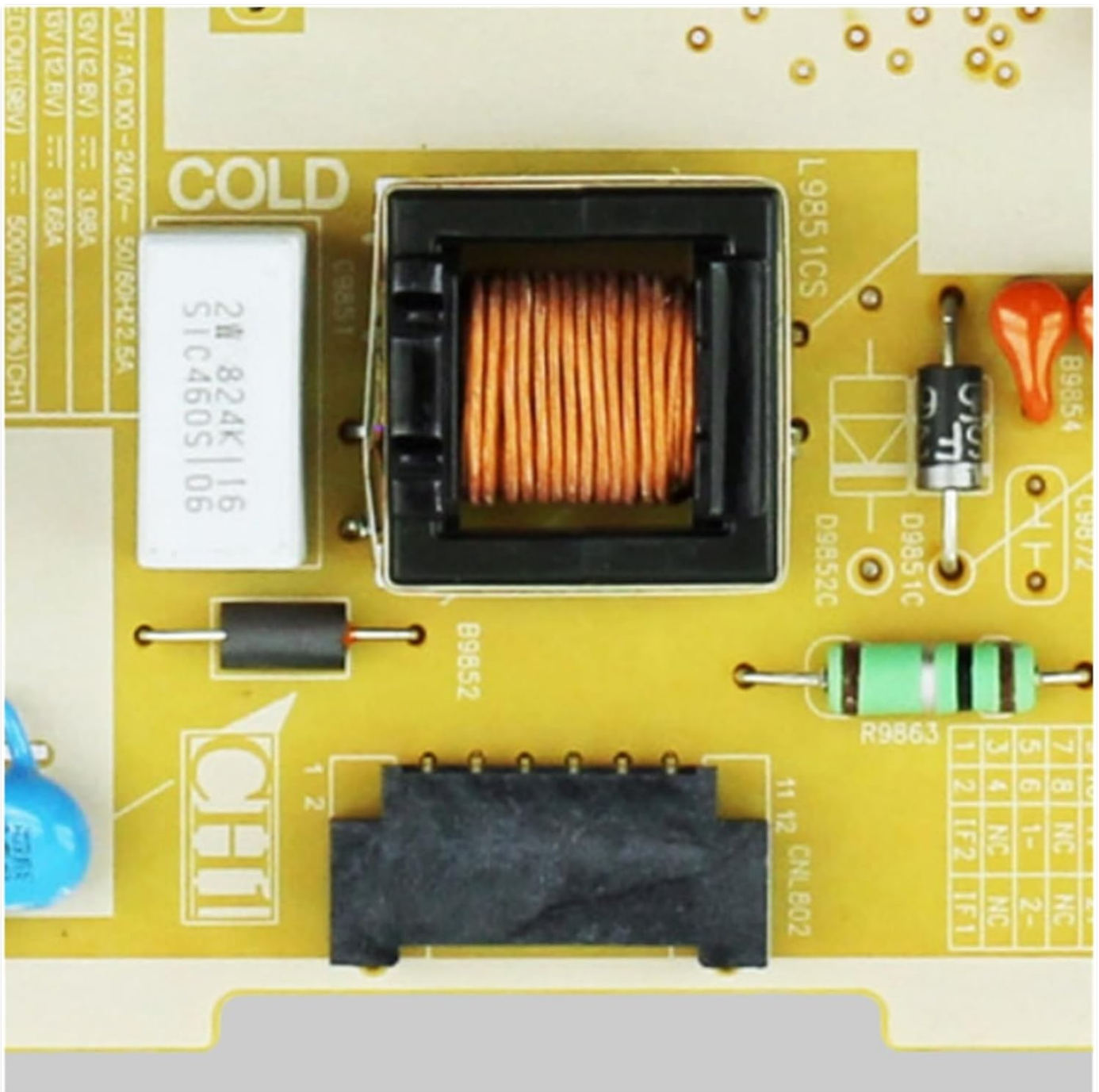
Image 5.1: A close-up view of a transformer (L9851CS) and surrounding components on the power supply board, which are integral to the power conversion process.
