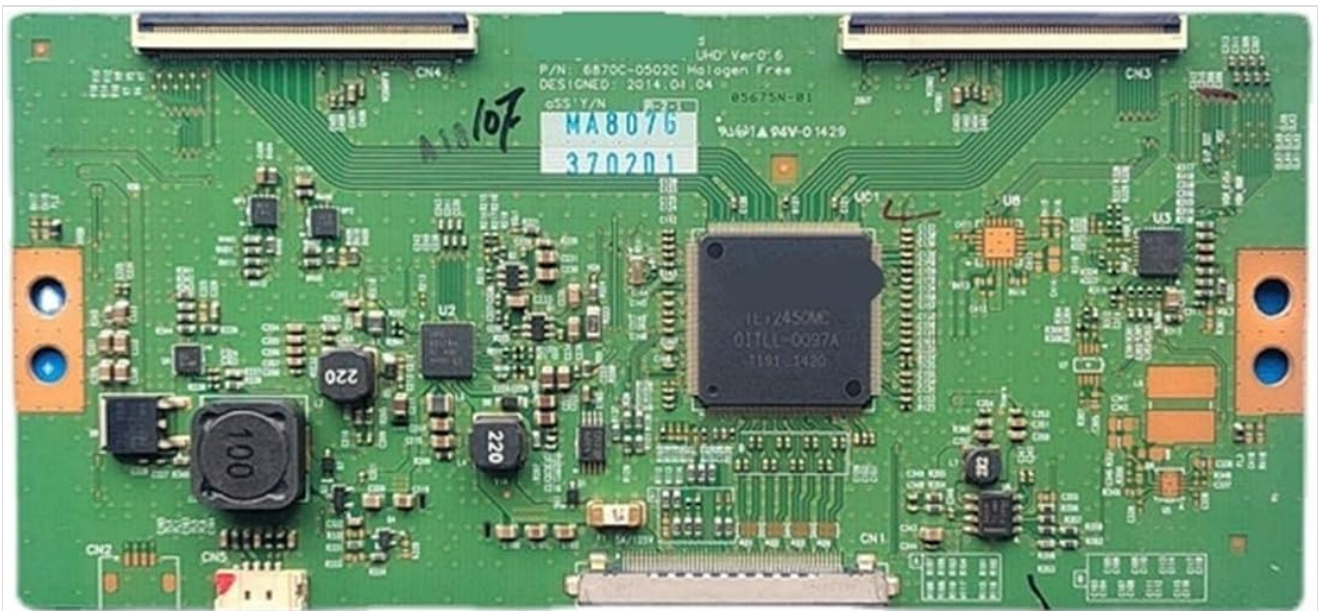
Figure 1: Top view of the T-CON board, illustrating component layout and connector locations.
