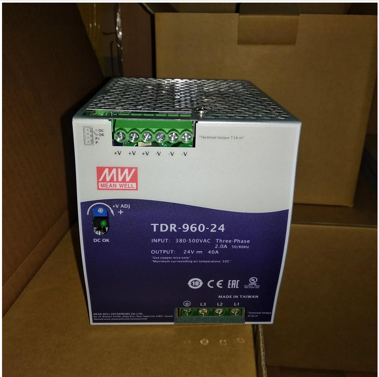
Figure 1: Front view of the TDR-960-24 power supply. Key features include the input terminals (L1, L2, L3, PE), output terminals (+V, -V), a DC OK indicator, and a +V ADJ potentiometer for output voltage adjustment. The label specifies 380-500VAC Three-Phase input and 24V 40A output.
