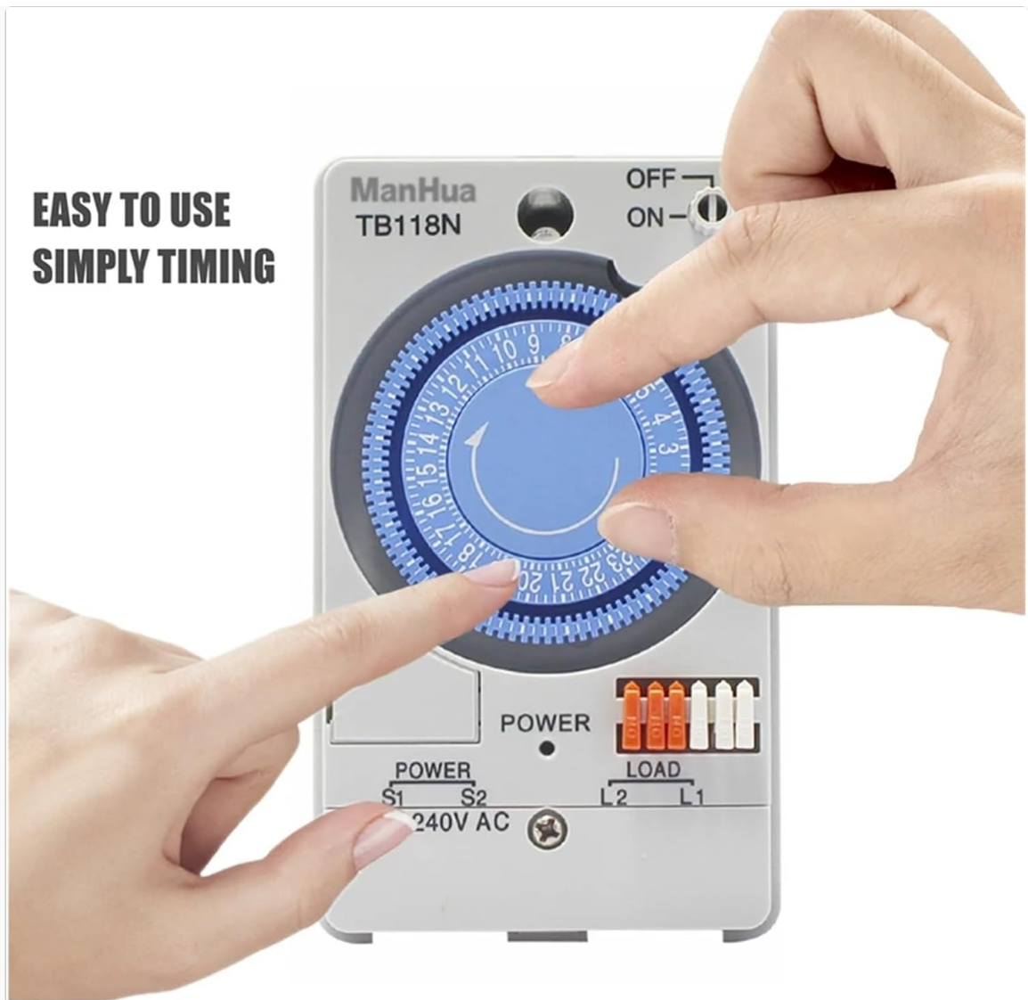
Figure 5: A hand demonstrating the adjustment of the dial plate for setting ON/OFF times. Pins are pushed out for ON periods and left in for OFF periods.
