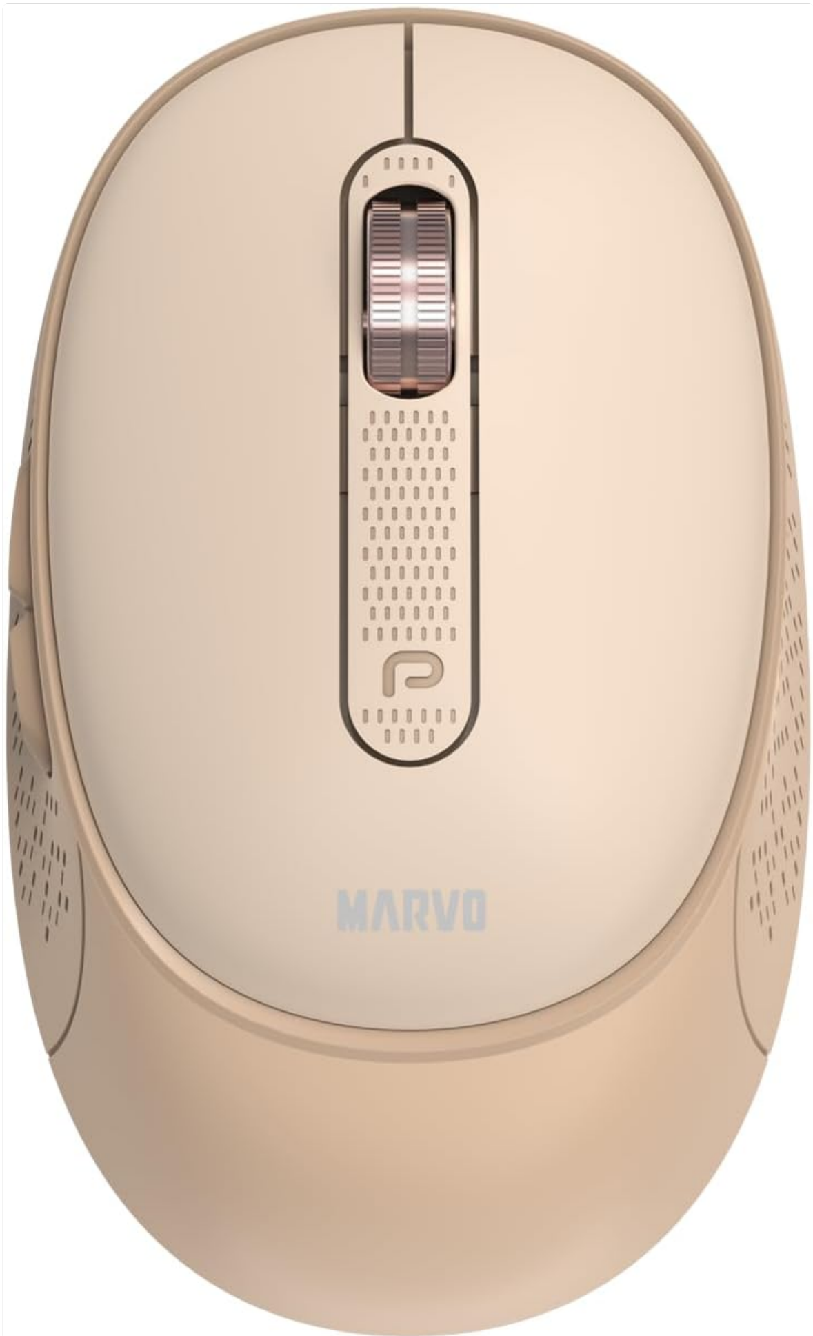
Figure 1: Top view of the MARVO WM111PK Wireless Mouse. This image displays the primary left and right click buttons, the central scroll wheel, and the MARVO branding.
