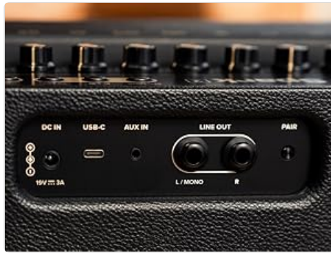
Figure 2: Rear panel connections of the Spark 2 Pearl amplifier.
