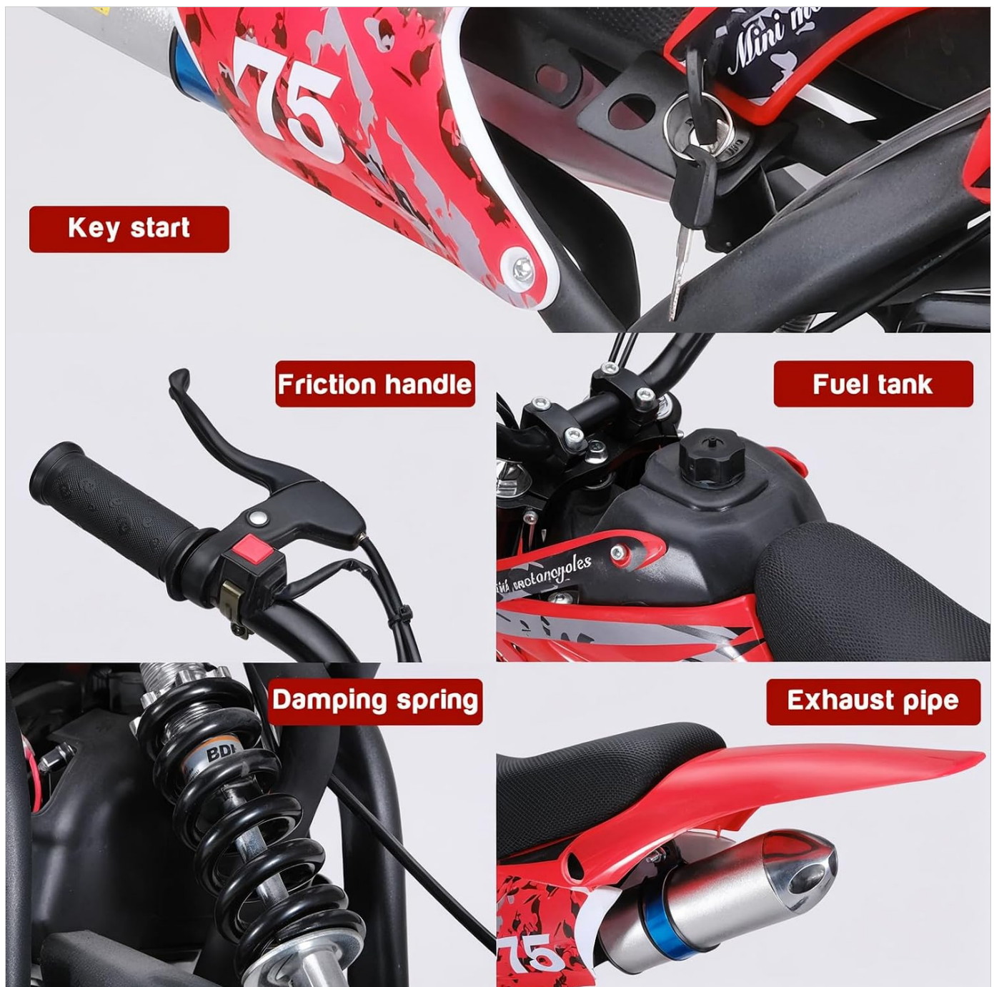
Figure 3.2: Close-up views of essential components including the key start ignition, friction handle (brake lever), fuel tank cap, rear damping spring, and exhaust pipe.
