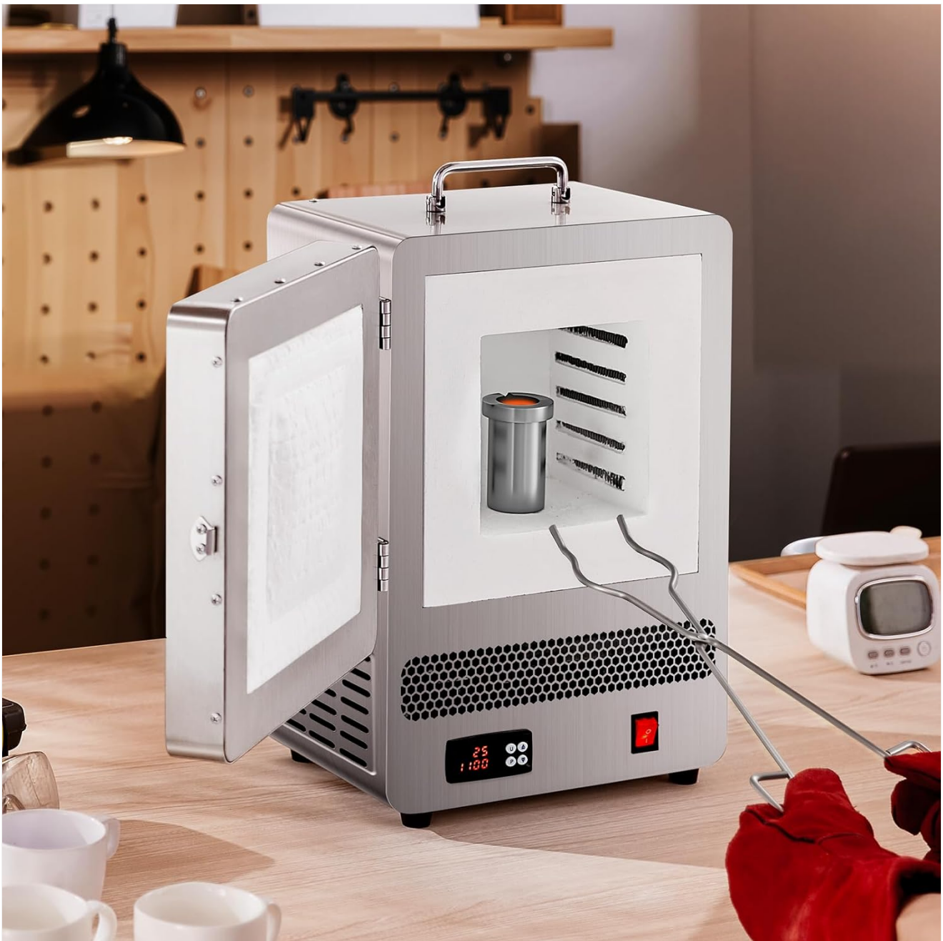
Figure 5: Proper technique for inserting a crucible into the kiln using the provided tongs and gloves.
