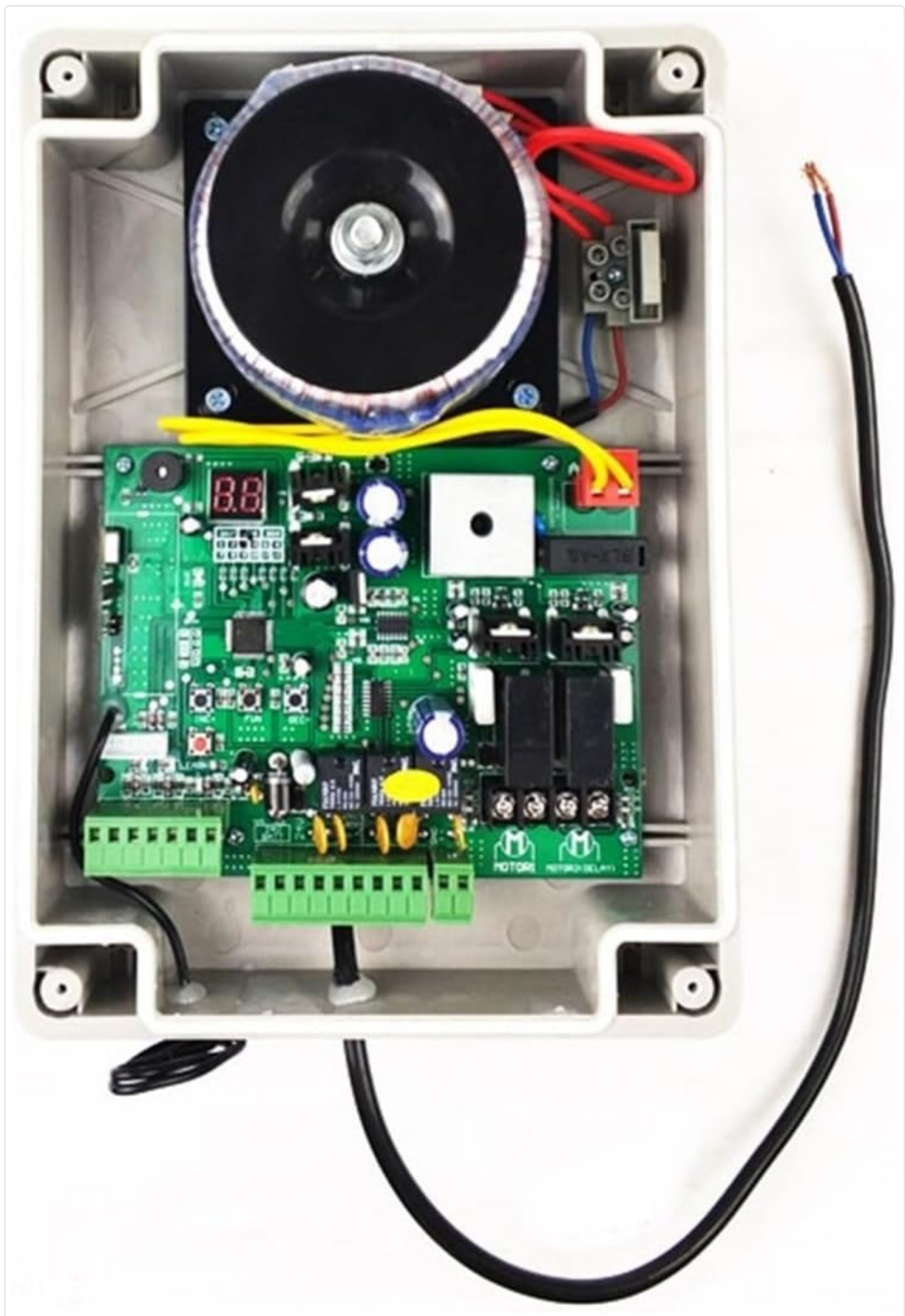
Image 2.3: The control board typically installed within a protective enclosure, demonstrating a common setup with a transformer.
