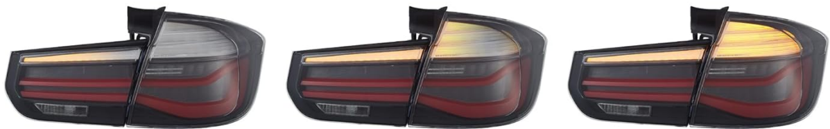
Image 6.2: Sequential turn signal indicator.
