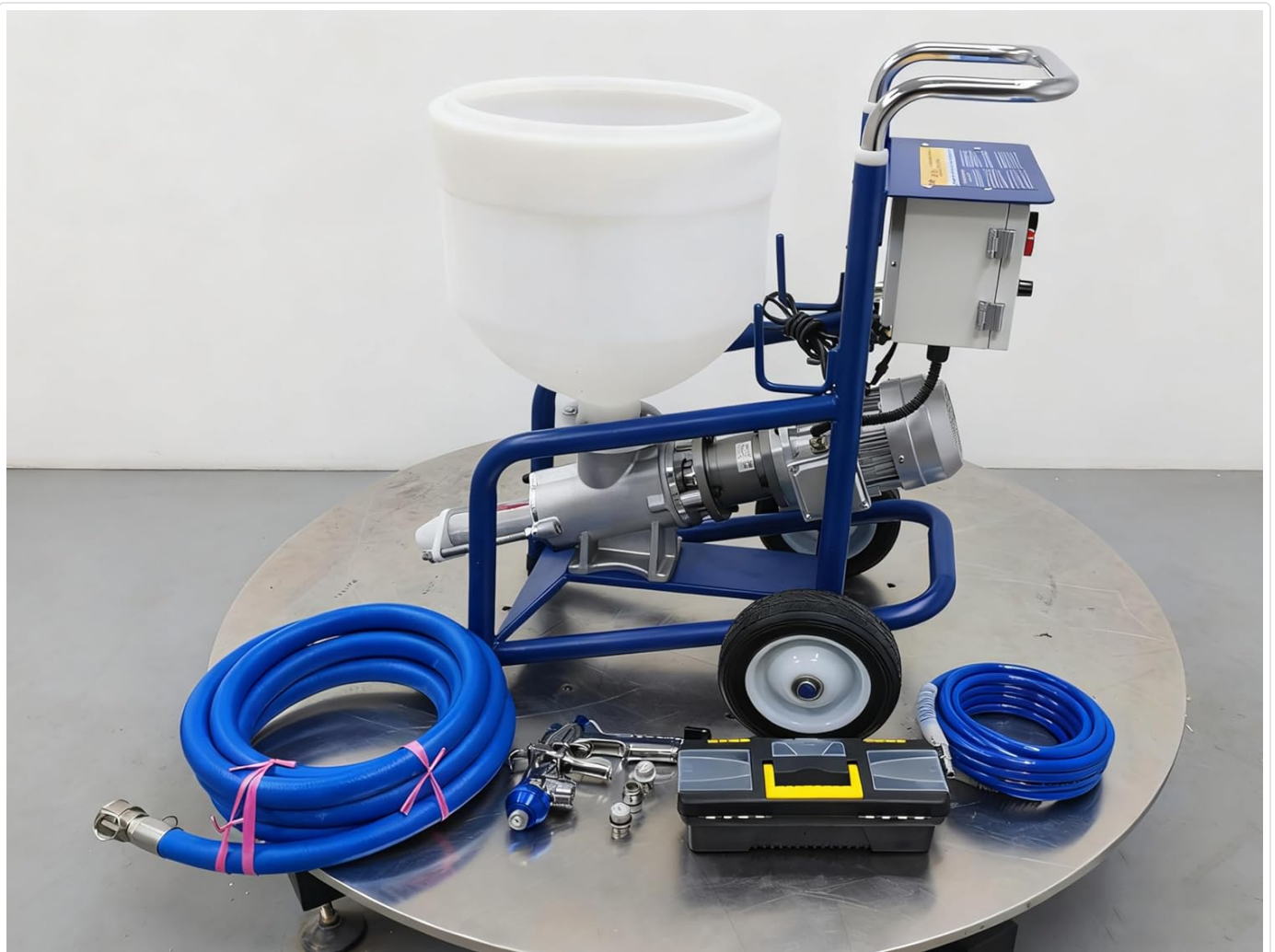
Figure 5: The sprayer unit alongside its standard accessories, including hoses, various nozzles, and a toolbox for maintenance.
