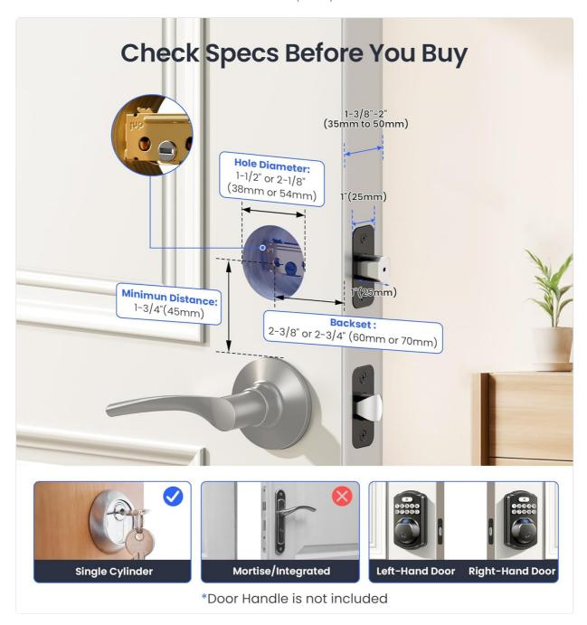
Text description: Diagram illustrating door measurements required for installation, including hole diameter, backset, bore diameter, and door thickness.
