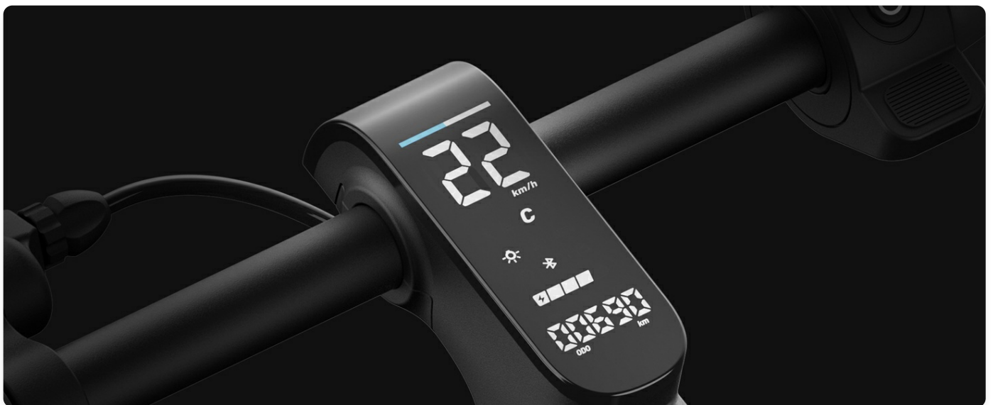
Image: A close-up of the scooter's LED dashboard, showing real-time speed, battery level, and trip information.
