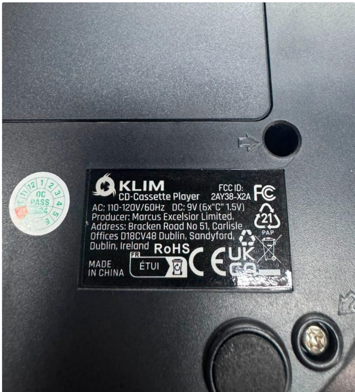
Figure 4.3: Product label on the bottom of the unit, indicating model number and electrical ratings.
