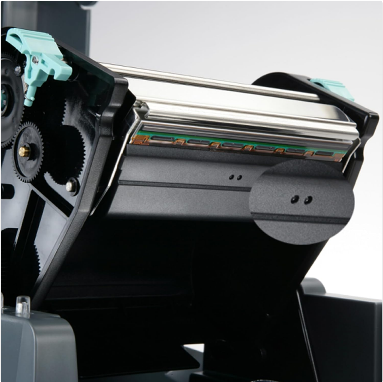
Image 5.1: A close-up view of the printer's internal print head and roller mechanism, highlighting areas that may require cleaning.
