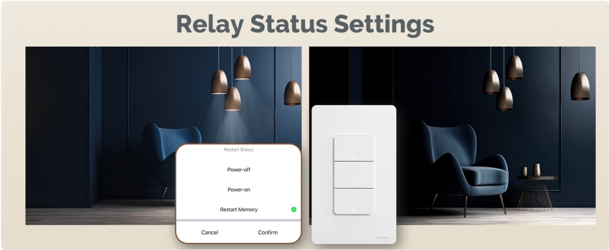
Image 4.6: Screenshot of the app interface for configuring relay status settings after a power interruption.
