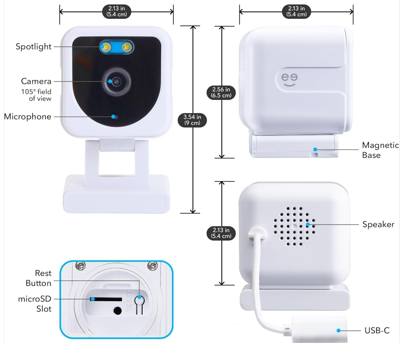
Image: Detailed dimensions and component labels of the Geeni Mini Camera.
